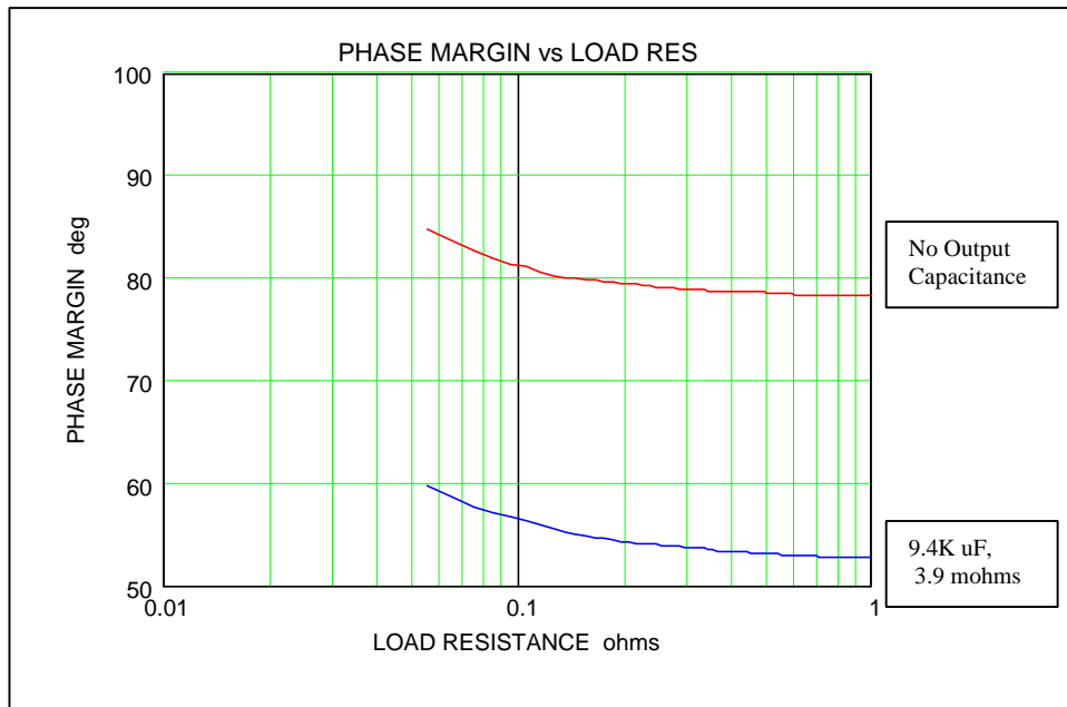
Figure 22: Phase Margin vs Load Resistance
